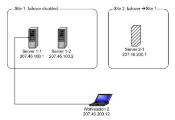
After Server 2-1 becomes available again, the existing session on Workstation 2 does not immediately fail back. Once the user locks and unlocks, or logs out and logs back in, a new connection is established within Site 2, as it is the home site for Workstation 2.
